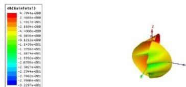
Fig.9b. The Simulated 3 dB gain pattern for  $\alpha = 60^0$
