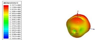
Fig.9c.The Simulated 3 dB gain pattern for  $\alpha = 90^0$
